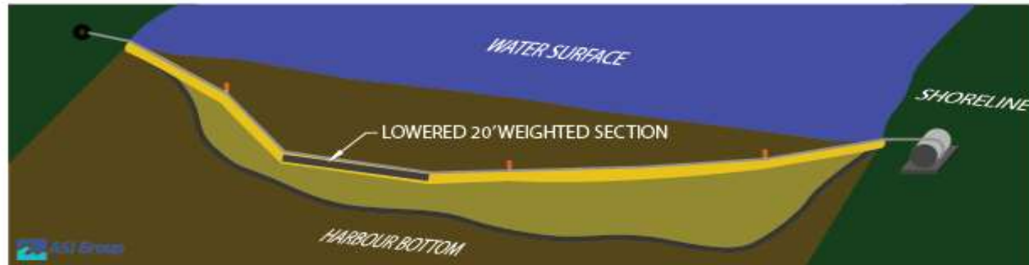
TYPICAL SILT CURTAIN LOWERED
